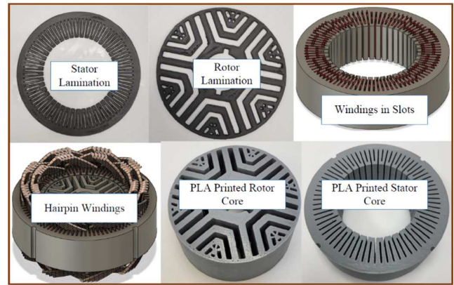
Fig. 11. Prototyping of a PMA SynRM
